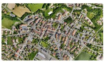
Create orthomosaics that are geometrically corrected such that the scale is uniform. They are color balanced in order to be visually pleasing.
